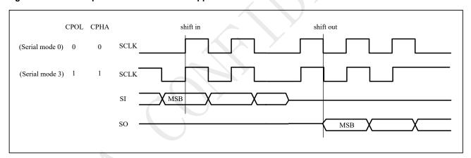
Figure 8-1 Serial Peripheral Interface Modes Supported
