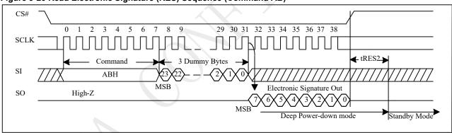
Figure 9-20a Release from Deep Power-down (RDP) Sequence (Command AB)
