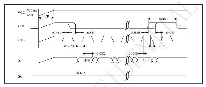
Figure 5-9 Power-up Timing
